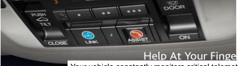
Your vehicle constantly monitors critical telemetry like airbag status, GPS location and – most critically – collision sensor activity. If an airbag ever deploys, the vehicle automatically sends an event report to AcuraLink support.
